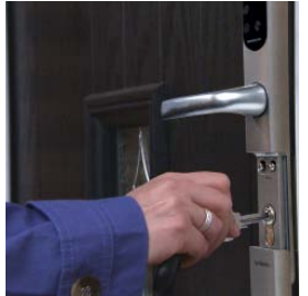
Keyfree is also fitted with a mechanical lock and key as a safety over-ride feature.
